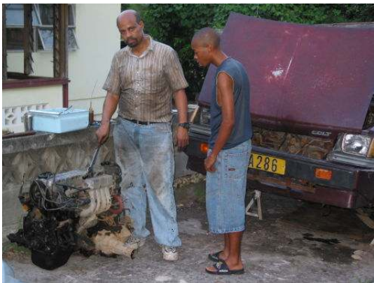
Walter and Jeshua observing the Vista's engine and transaxle after removing it from the chassis
