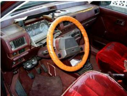
(Left) The Vista interior is cracking and falling apart.
